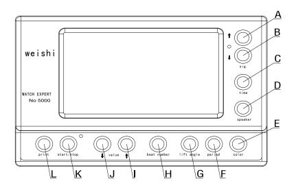
Signal↑ The key used for increase the signal А В The key used for decrease the signal Signal↓ С Clock The key used for adjust the build in clock D Speaker The key used for turn on/off the speaker Е Color The key used for adjust the display color F Period The key used for the test period Lift Angle The key used for adjustment the lift angle G н Beat Number The key used for adjustment the beat number L The key used for selection of the next higher value Value↑
